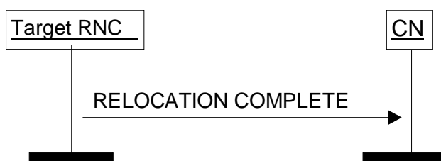
Figure 10: Relocation Complete procedure. Successful operation.
