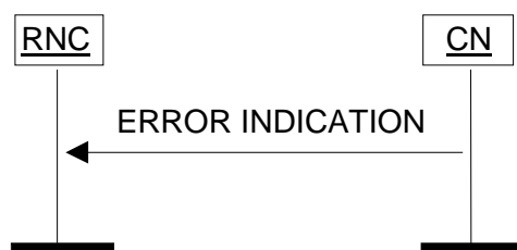
Figure 31: Error Indication procedure, CN originated. Successful operation.
