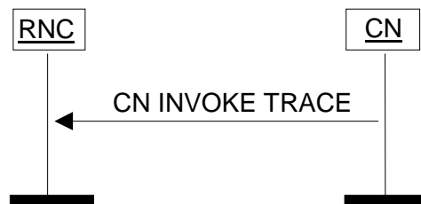
Figure 18: CN Invoke Trace procedure. Successful operation.
