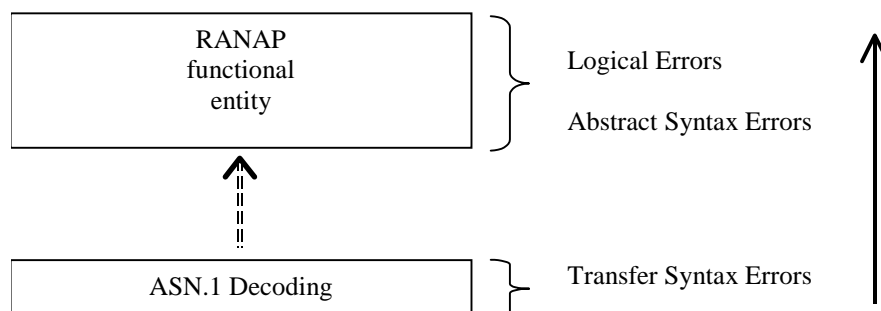
Figure 36: Protocol Errors in RANAP.
