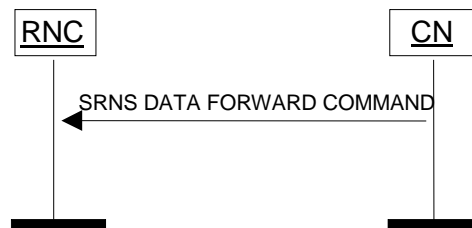
Figure 13: SRNS Data Forwarding Initiation procedure. Successful operation.
