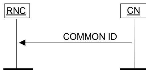
Figure 17: Common ID procedure. Successful operation.
