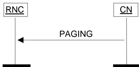
Figure 16: Paging procedure. Successful operation.
