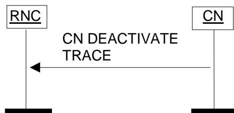
Figure 33: CN Deactivate Trace procedure. Successful operation.
