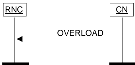
Figure 27: Overload at the CN. Successful operation.
