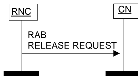
Figure 2: RAB Release Request procedure. Successful operation.
