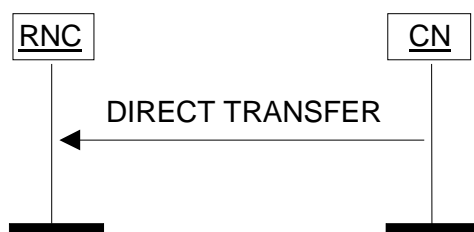
Figure 25: Direct Transfer, CN originated. Successful operation.
