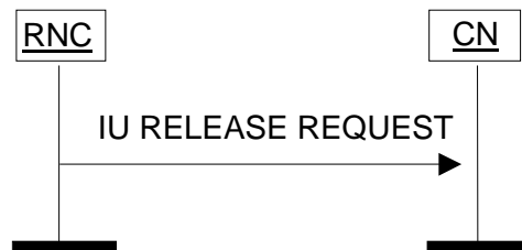
Figure 3: Iu Release Request procedure. Successful operation.
