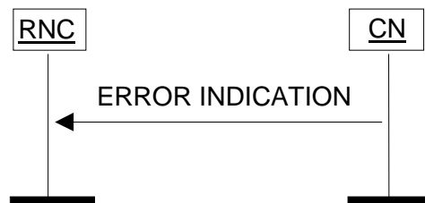
Figure 31: Error Indication procedure, CN originated. Successful operation.
