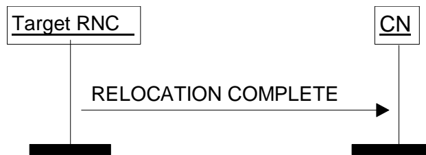
Figure 10: Relocation Complete procedure. Successful operation.
