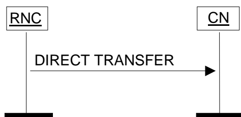
Figure 26: Direct Transfer, RNC originated. Successful operation.
