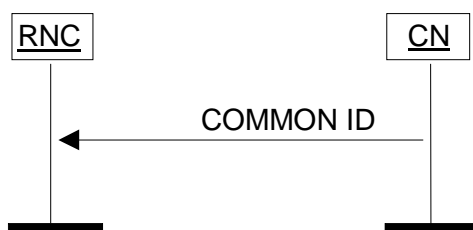
Figure 17: Common ID procedure. Successful operation.
