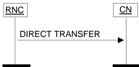
Figure 26: Direct Transfer, RNC originated. Successful operation.
