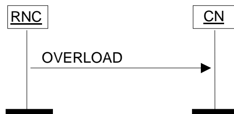
Figure 28: Overload at the UTRAN. Successful operation.
