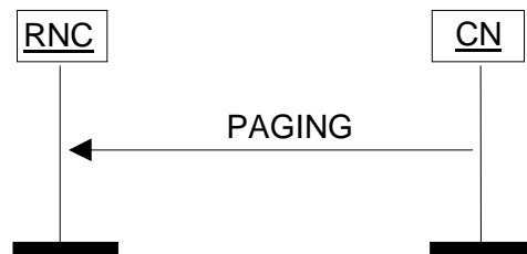
Figure 16: Paging procedure. Successful operation.
