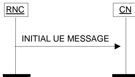
Figure 24: Initial UE Message procedure. Successful operation.
