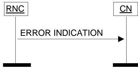
Figure 32: Error Indication procedure, RNC originated. Successful operation.
