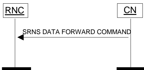
Figure 13: SRNS Data Forwarding Initiation procedure. Successful operation.
