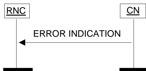
Figure 31: Error Indication procedure, CN originated. Successful operation.
