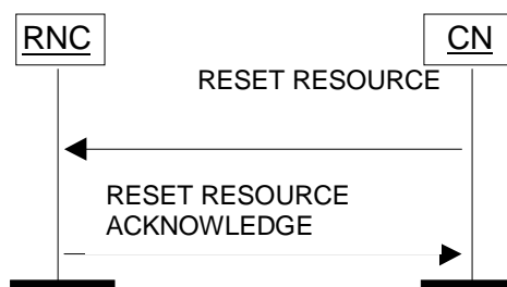
Figure 35: CN initiated Reset Resource procedure. Successful operation.
