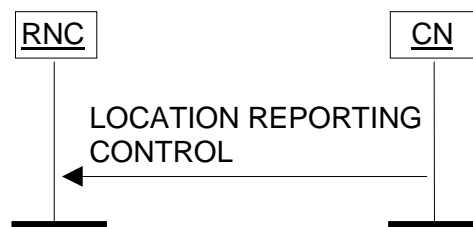
Figure 21: Location Reporting Control procedure. Successful operation.
