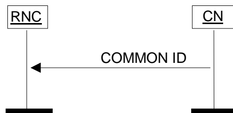
Figure 17: Common ID procedure. Successful operation.
