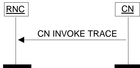
Figure 18: CN Invoke Trace procedure. Successful operation.
