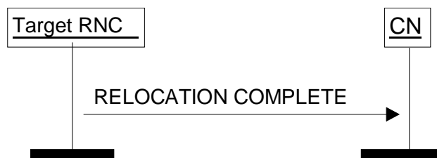
Figure 10: Relocation Complete procedure. Successful operation.
