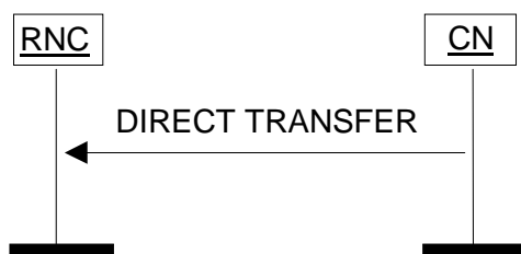
Figure 25: Direct Transfer, CN originated. Successful operation.
