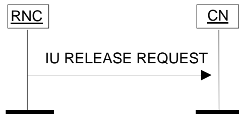
Figure 3: Iu Release Request procedure. Successful operation.
