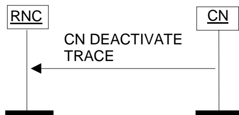
Figure 33: CN Deactivate Trace procedure. Successful operation.
