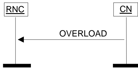
Figure 27: Overload at the CN. Successful operation.
