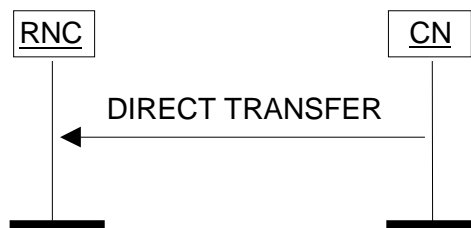
Figure 25: Direct Transfer, CN originated. Successful operation.
