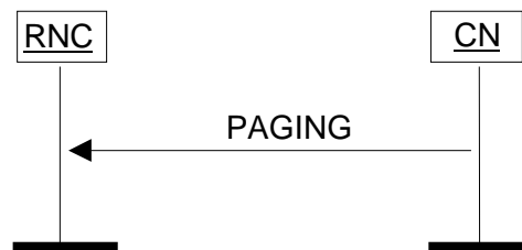
Figure 16: Paging procedure. Successful operation.
