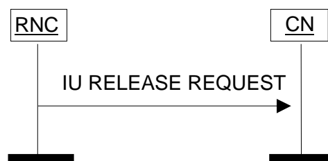
Figure 3: Iu Release Request procedure. Successful operation.
