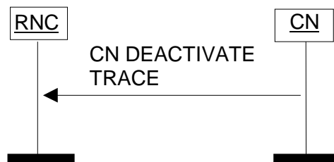
Figure 33: CN Deactivate Trace procedure. Successful operation.
