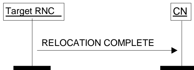
Figure 10: Relocation Complete procedure. Successful operation.
