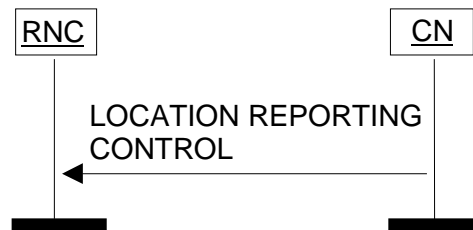
Figure 21: Location Reporting Control procedure. Successful operation.
