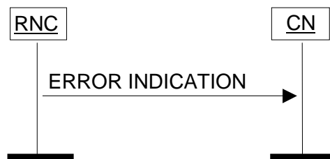
Figure 32: Error Indication procedure, RNC originated. Successful operation.
