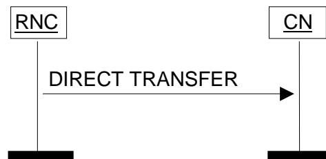
Figure 26: Direct Transfer, RNC originated. Successful operation.
