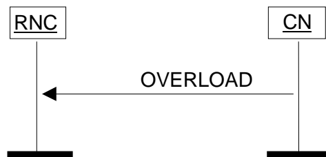
Figure 27: Overload at the CN. Successful operation.
