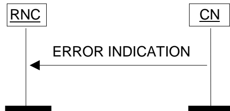
Figure 31: Error Indication procedure, CN originated. Successful operation.
