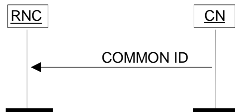
Figure 17: Common ID procedure. Successful operation.
