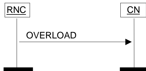
Figure 28: Overload at the UTRAN. Successful operation.
