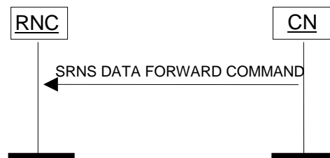
Figure 13: SRNS Data Forwarding Initiation procedure. Successful operation.
