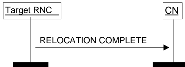
Figure 10: Relocation Complete procedure. Successful Operation
