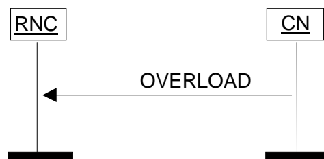
Figure 29: Overload at the CN
