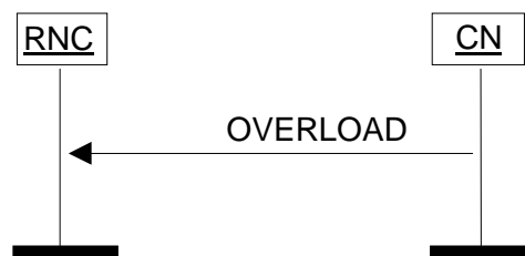
Figure 29: Overload at the CN.
