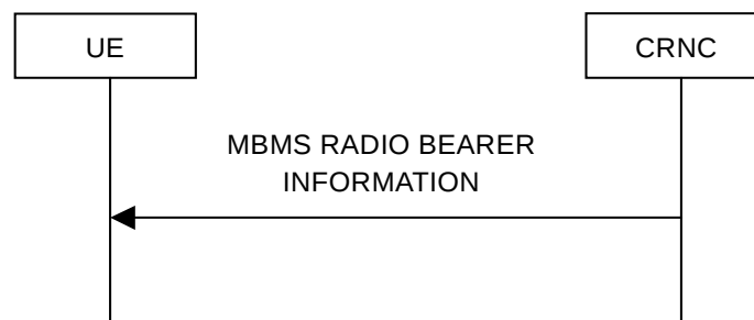
Figure 8.3.3: MBMS radio bearer information signalling flow
