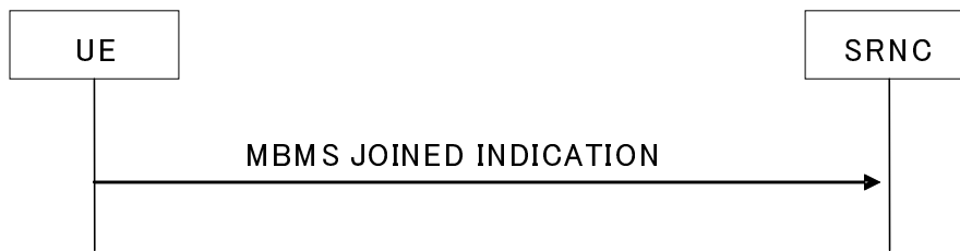
Figure 8.3.6: MBMS joined indication signalling flow
