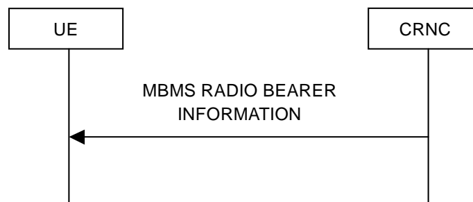
Figure 8.3.3: MBMS radio bearer information signalling flow
