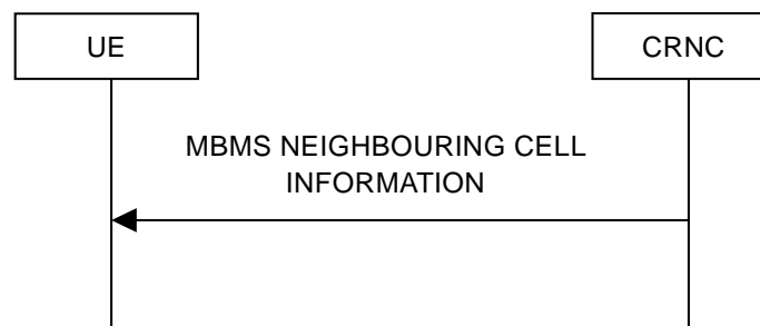
Figure 8.3.5: MBMS Neighbouring Cell Information signalling flow
