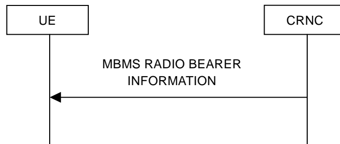
Figure 8.3.3: MBMS radio bearer information signalling flow
