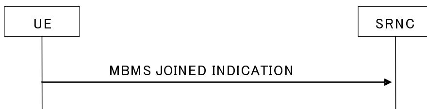
Figure 8.3.6: MBMS joined indication signalling flow
