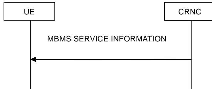
Figure 8.3.2: MBMS service information signalling flow
