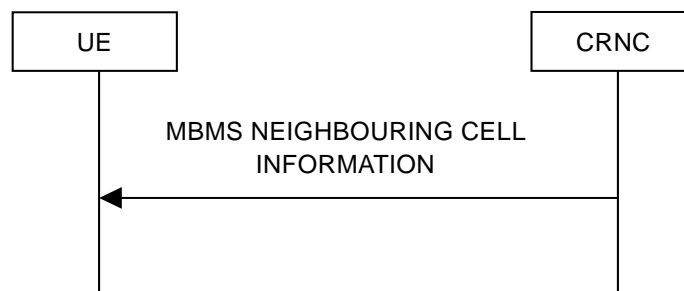
Figure 8.3.5: MBMS Neighbouring Cell Information signalling flow
