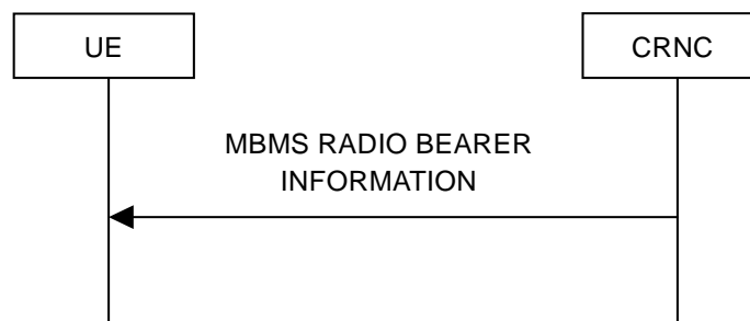
Figure 8.3.3: MBMS radio bearer information signalling flow
