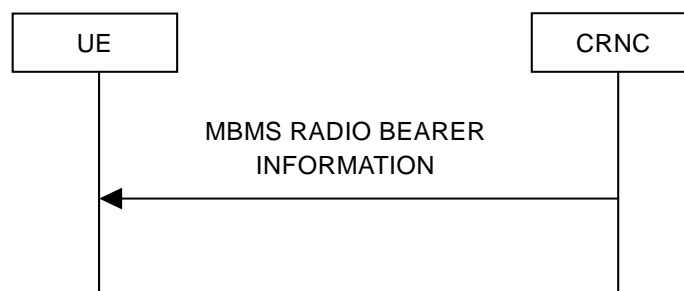
Figure 8.3.3: MBMS radio bearer information signalling flow
