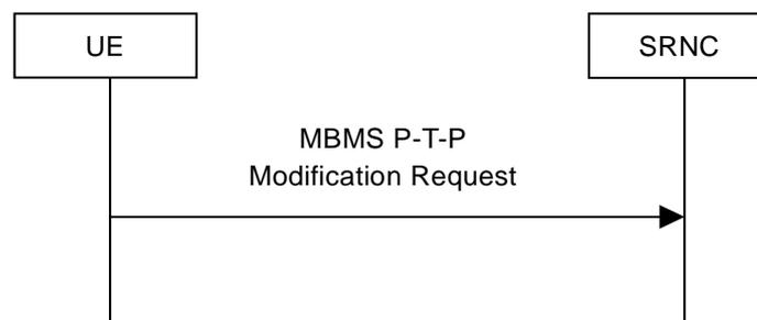
**Figure 8.3.9: MBMS P-T-P Modification Request.**
