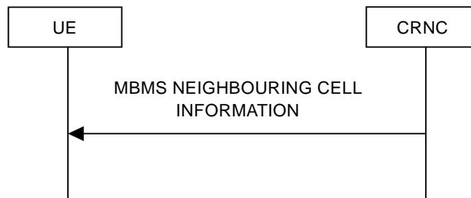
**Figure 8.3.5: MBMS Neighbouring Cell Information signalling flow**
