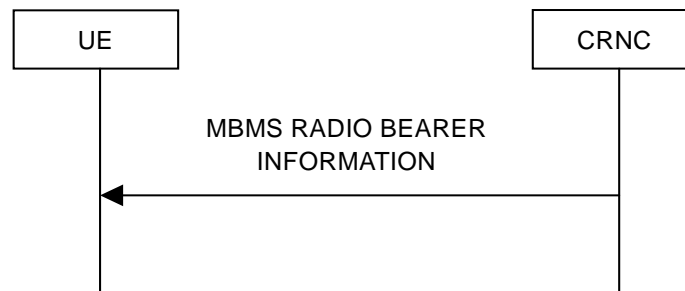
Figure 8.3.3: MBMS radio bearer information signalling flow
