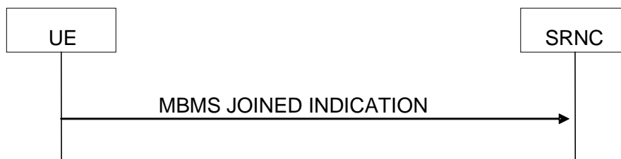
Figure 8.3.6: MBMS joined indication signalling flow
