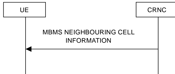
Figure 8.3.5: MBMS Neighbouring Cell Information signalling flow
