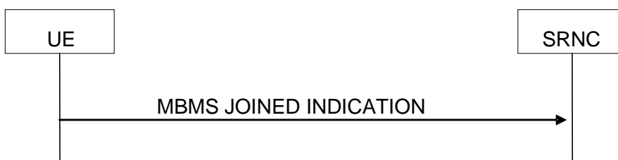
Figure 8.3.6: MBMS joined indication signalling flow
