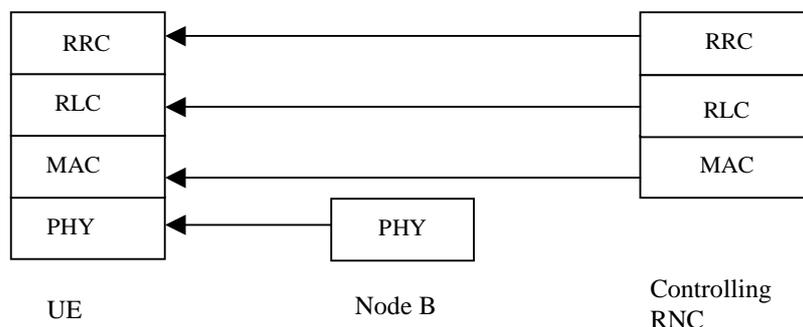
**Figure 5.3.2: Protocol Stack for MCCH and MSCH**
