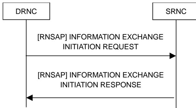
**Figure 8.2.13: Information Exchange Initiation signalling flow: Successful Operation.**
