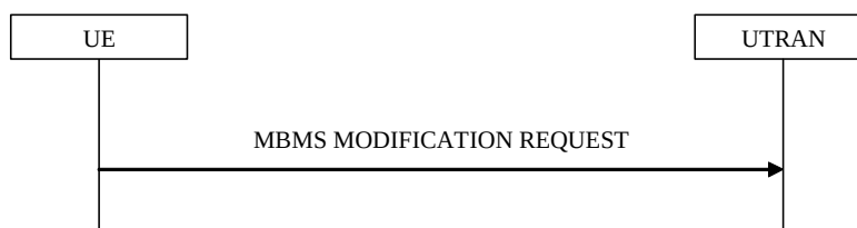
Figure 8.7.6-1: MBMS modification request, normal
