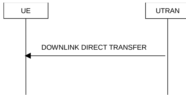
Figure 8.1.9-1: Downlink Direct transfer, normal flow
