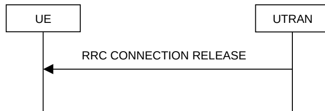
Figure 8.1.4-2: RRC Connection Release procedure on the CCCH
