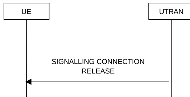
Figure 8.1.13-1: Signalling connection release procedure, normal case
