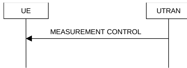
Figure 8.4.1-1: Measurement Control, normal case
