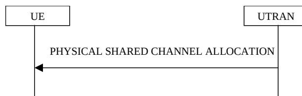
Figure 8.2.7-1: Physical Shared Channel Allocation
