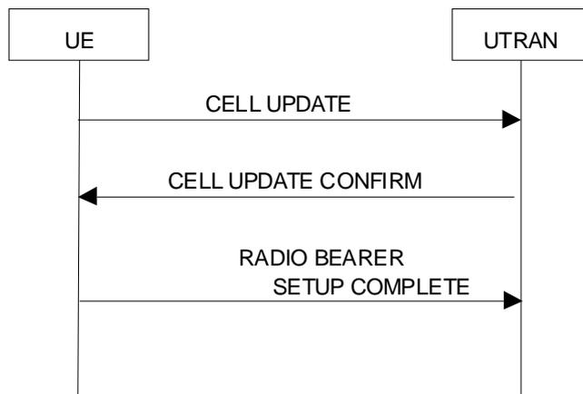
**Figure 8.3.1-6a: Cell update procedure with radio bearer setup**
