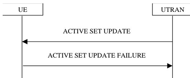
**Figure 8.3.4-2: Active Set Update procedure, failure case**
