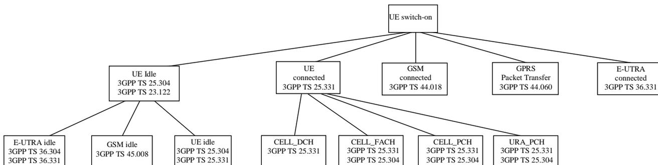
Figure 4.1-1: Mapping of UE state to 3GPP Specifications
