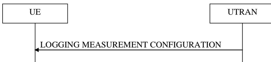
**Figure 8.5.63.1-1: Logged measurements configuration**
