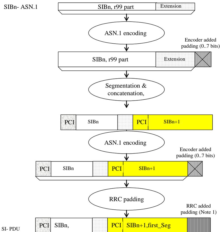
Note 1: RRC padding needs to be added only to octet align BCCH blocks which are mapped onto HS-DSCH
