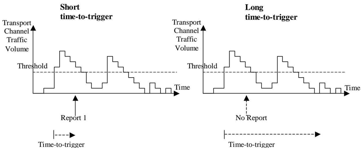
**Figure 14.4.3.1-2: Time-to-trigger is used to achieve time hysteresis**
