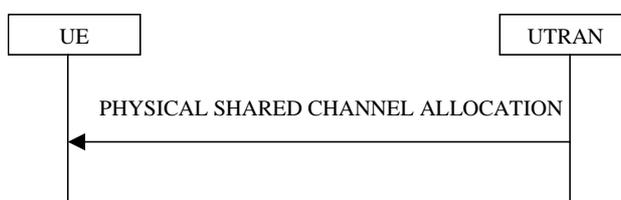
Figure 8.2.7-1: Physical Shared Channel Allocation
