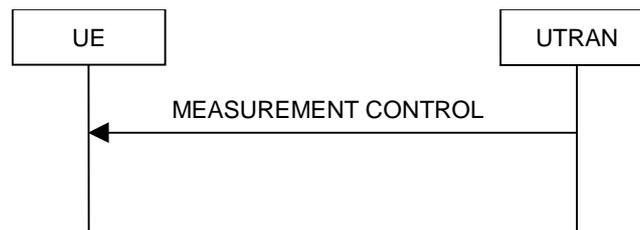
Figure 8.4.1-1: Measurement Control, normal case
