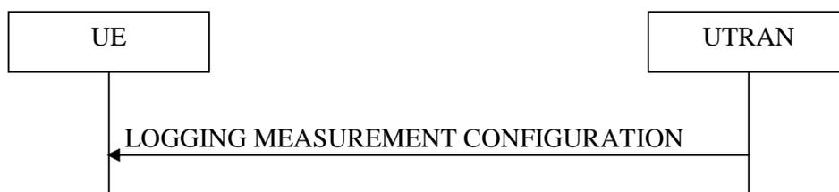
**Figure 8.5.63.1-1: Logged measurements configuration**
