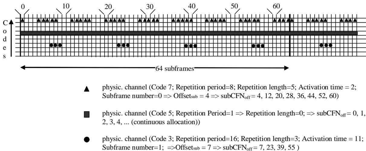
Figure 8.6.6.16a-1: Examples for subframe allocations in TDD
