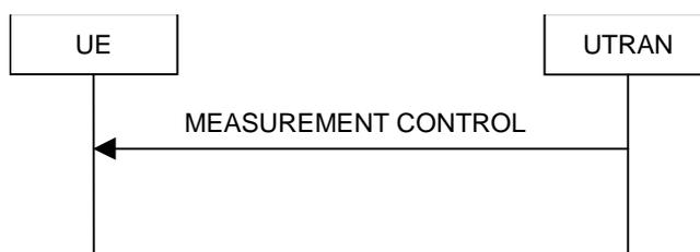
Figure 8.4.1-1: Measurement Control, normal case
