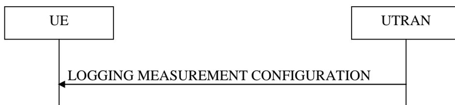
**Figure 8.5.63.1-1: Logged measurements configuration**
