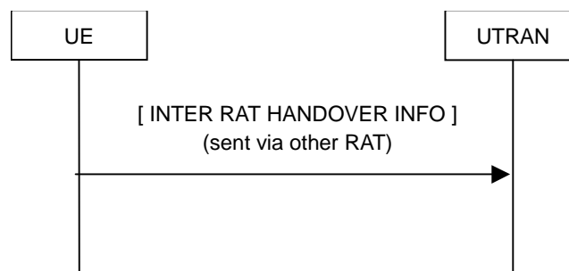
Figure 8.1.16-1: Inter RAT handover information transfer, normal flow
