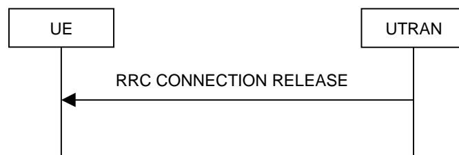
Figure 8.1.4-2: RRC Connection Release procedure on the CCCH
