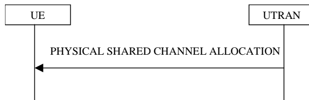
Figure 8.2.7-1: Physical Shared Channel Allocation
