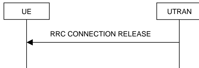
Figure 8.1.4-2: RRC Connection Release procedure on the CCCH
