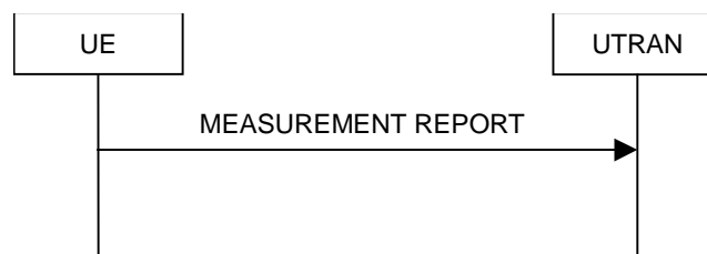
Figure 8.4.2-1: Measurement report, normal case
