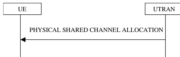
Figure 8.2.7-1: Physical Shared Channel Allocation
