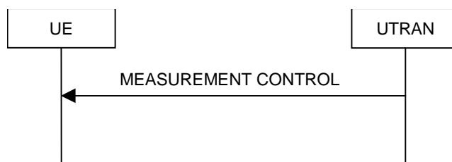
Figure 8.4.1-1: Measurement Control, normal case
