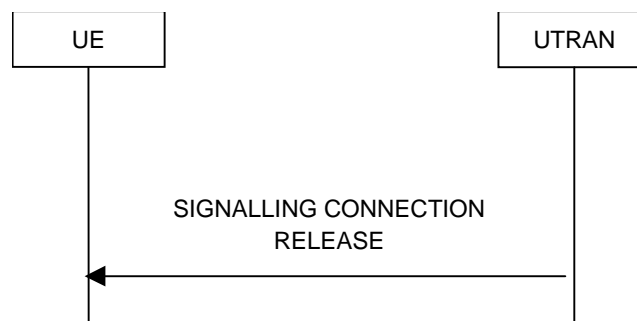
Figure 8.1.13-1: Signalling connection release procedure, normal case
