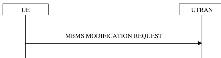
Figure 8.7.6-1: MBMS modification request, normal
