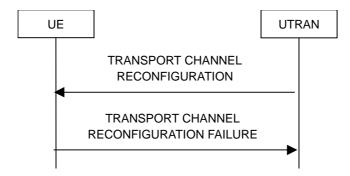
Figure 8.2.2-8: Transport channel reconfiguration, failure case
