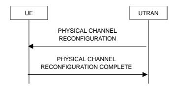
Figure 8.2.2-9: Physical channel reconfiguration, normal flow
