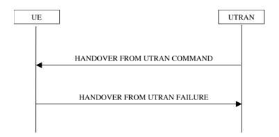
Figure 8.3.7-2: Inter-RAT handover from UTRAN, failure case
