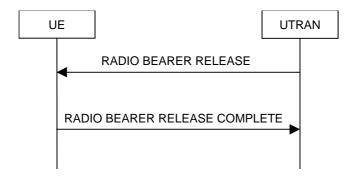
Figure 8.2.2-5: Radio Bearer Release, normal case
