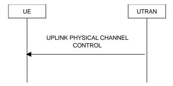
Figure 8.2.10-1: Uplink Physical Channel Control
