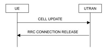
Figure 8.3.1-7: Cell update procedure, failure case
