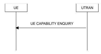
Figure 8.1.7-1: UE capability enquiry procedure, normal flow
