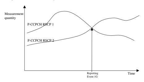
Figure 14.1.3.1-1: A P-CCPCH RSCP becomes better than the previous best P-CCPCH RSCP
