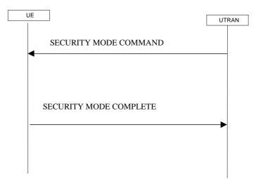
Figure 8.1.12-1: Security mode control procedure
