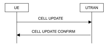
Figure 8.3.1-1: Cell update procedure, basic flow
