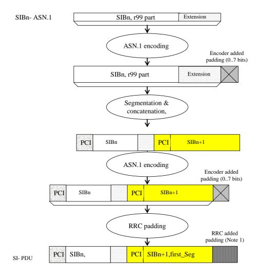
Note 1: RRC padding needs to be added only to octet align BCCH blocks which are mapped onto HS-DSCH
