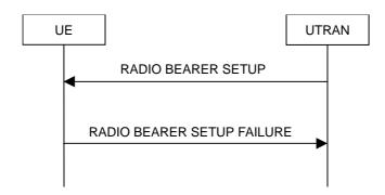
Figure 8.2.2-2: Radio Bearer Establishment, failure case
