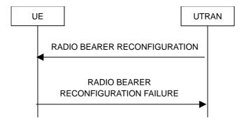
Figure 8.2.2-4: Radio bearer reconfiguration, failure case
