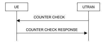
Figure 8.1.15-1: Counter check procedure
