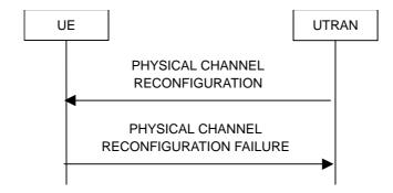
Figure 8.2.2-10: Physical channel reconfiguration, failure case
