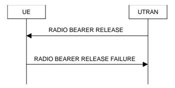
Figure 8.2.2-6: Radio Bearer Release, failure case
