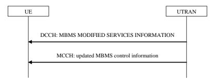
Figure 8.7.3-2: MBMS notification on DCCH
