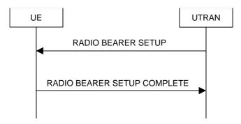
Figure 8.2.2-1: Radio Bearer Establishment, normal case
