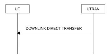
Figure 8.1.9-1: Downlink Direct transfer, normal flow
