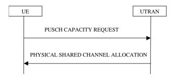
Figure 8.2.8-1: PUSCH Capacity request procedure
