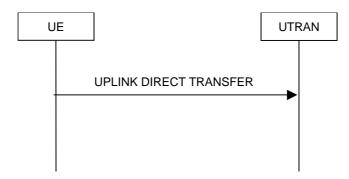
Figure 8.1.10-1: Uplink Direct transfer, normal flow
