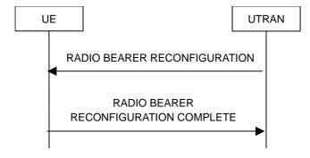
Figure 8.2.2-3: Radio bearer reconfiguration, normal flow
