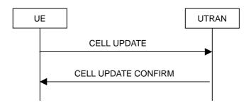
Figure 8.3.1-1: Cell update procedure, basic flow
