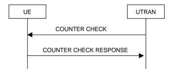
Figure 8.1.15-1: Counter check procedure
