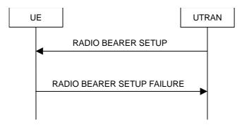
Figure 8.2.2-2: Radio Bearer Establishment, failure case
