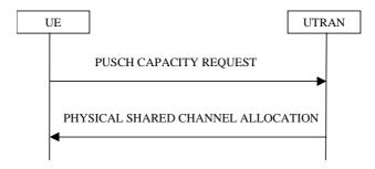
Figure 8.2.8-1: PUSCH Capacity request procedure
