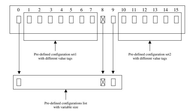
Figure C.2-2: Example scenario where non-stored pre-defined configurations need to be explicitly indicated
