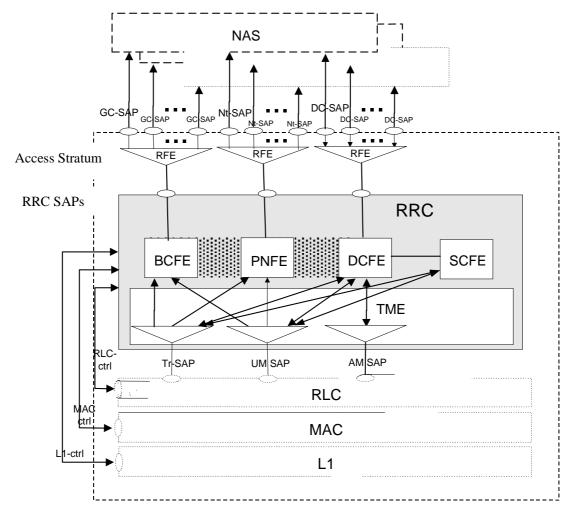
Figure 4.2-1: UE side model of RRC
