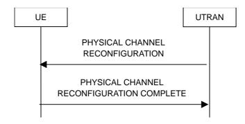
Figure 8.2.2-9: Physical channel reconfiguration, normal flow
