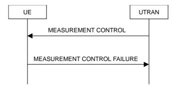
Figure 8.4.1-2: Measurement Control, failure case
