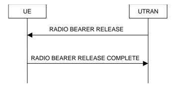
Figure 8.2.2-5: Radio Bearer Release, normal case
