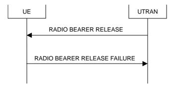
Figure 8.2.2-6: Radio Bearer Release, failure case
