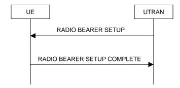
Figure 8.2.2-1: Radio Bearer Establishment, normal case
