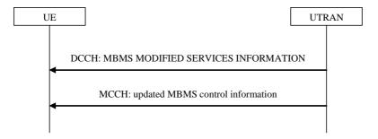
Figure 8.7.3-2: MBMS notification on DCCH
