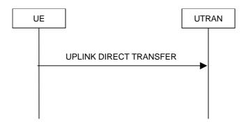
Figure 8.1.10-1: Uplink Direct transfer, normal flow
