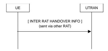
Figure 8.1.16-1: Inter RAT handover information transfer, normal flow
