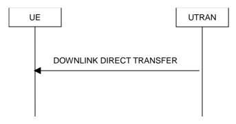
Figure 8.1.9-1: Downlink Direct transfer, normal flow
