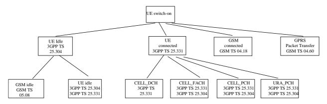
Figure 4.1-1: Mapping of UE state to 3GPP Specifications
