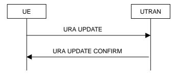
Figure 8.3.1-8: URA update procedure, basic flow
