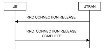
Figure 8.1.4-1: RRC Connection Release procedure on the DCCH
