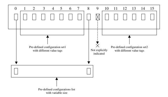
Figure C.2-1: Example scenario where non-stored pre-defined configurations do not need to be explicitly indicated
