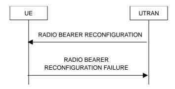
Figure 8.2.2-4: Radio bearer reconfiguration, failure case
