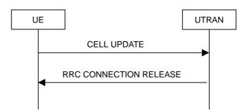
Figure 8.3.1-7: Cell update procedure, failure case
