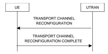
Figure 8.2.2-7: Transport channel reconfiguration, normal flow
