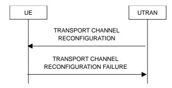
Figure 8.2.2-8: Transport channel reconfiguration, failure case
