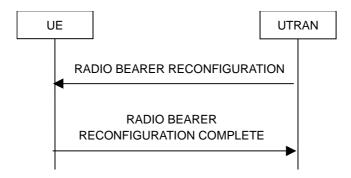
Figure 8.2.2-3: Radio bearer reconfiguration, normal flow
