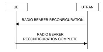
Figure 8.2.2-3: Radio bearer reconfiguration, normal flow
