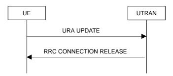
Figure 8.3.1-10: URA update procedure, failure case
