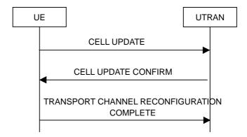
Figure 8.3.1-4: Cell update procedure with transport channel reconfiguration
