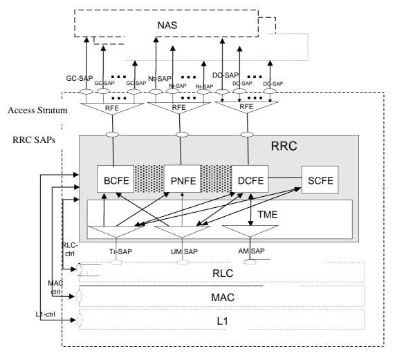
Figure 4.2-1: UE side model of RRC
