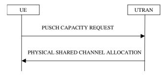
Figure 8.2.8-1: PUSCH Capacity request procedure
