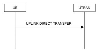
Figure 8.1.10-1: Uplink Direct transfer, normal flow
