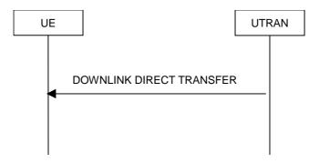
Figure 8.1.9-1: Downlink Direct transfer, normal flow
