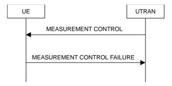
Figure 8.4.1-2: Measurement Control, failure case
