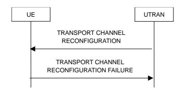
Figure 8.2.2-8: Transport channel reconfiguration, failure case
