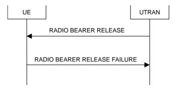
Figure 8.2.2-6: Radio Bearer Release, failure case
