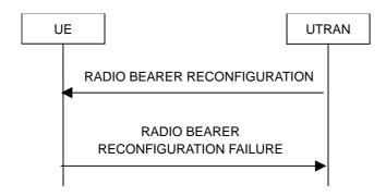
Figure 8.2.2-4: Radio bearer reconfiguration, failure case
