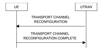
Figure 8.2.2-7: Transport channel reconfiguration, normal flow
