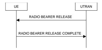
Figure 8.2.2-5: Radio Bearer Release, normal case
