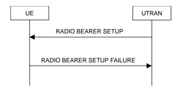
Figure 8.2.2-2: Radio Bearer Establishment, failure case
