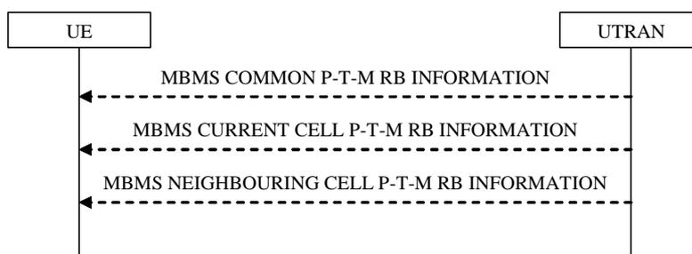
Figure 8.7.5-1: MBMS p-t-m radio bearer modification, normal
