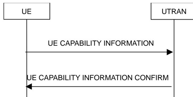
**Figure 8.1.6-1: Transmission of UE capability information, normal flow**
