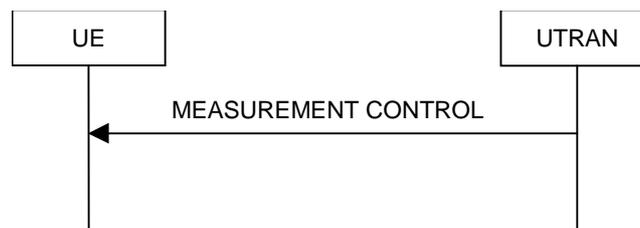
Figure 8.4.1-1: Measurement Control, normal case
