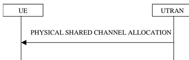
Figure 8.2.7-1: Physical Shared Channel Allocation
