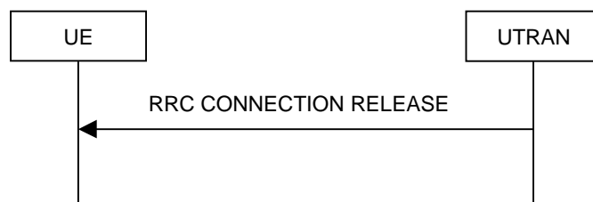
Figure 8.1.4-2: RRC Connection Release procedure on the CCCH
