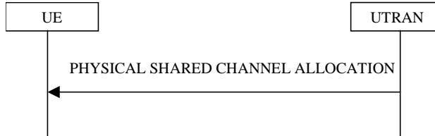
**Figure 8.2.7-1: Physical Shared Channel Allocation**
