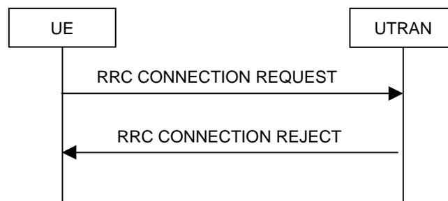
**Figure 8.1.3-2: RRC Connection Establishment, network rejects RRC connection**
