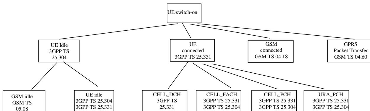
Figure 4.1-1: Mapping of UE state to 3GPP Specifications
