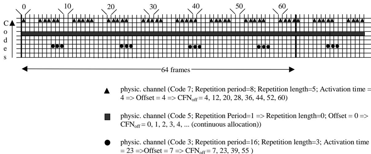
**Figure 8.6.6.16-1: Examples for frame allocations in TDD**
