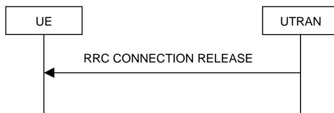
Figure 8.1.4-2: RRC Connection Release procedure on the CCCH
