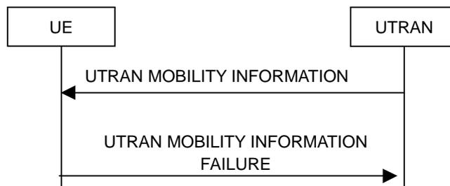
**Figure 8.3.3-2: UTRAN mobility information procedure, failure case**
