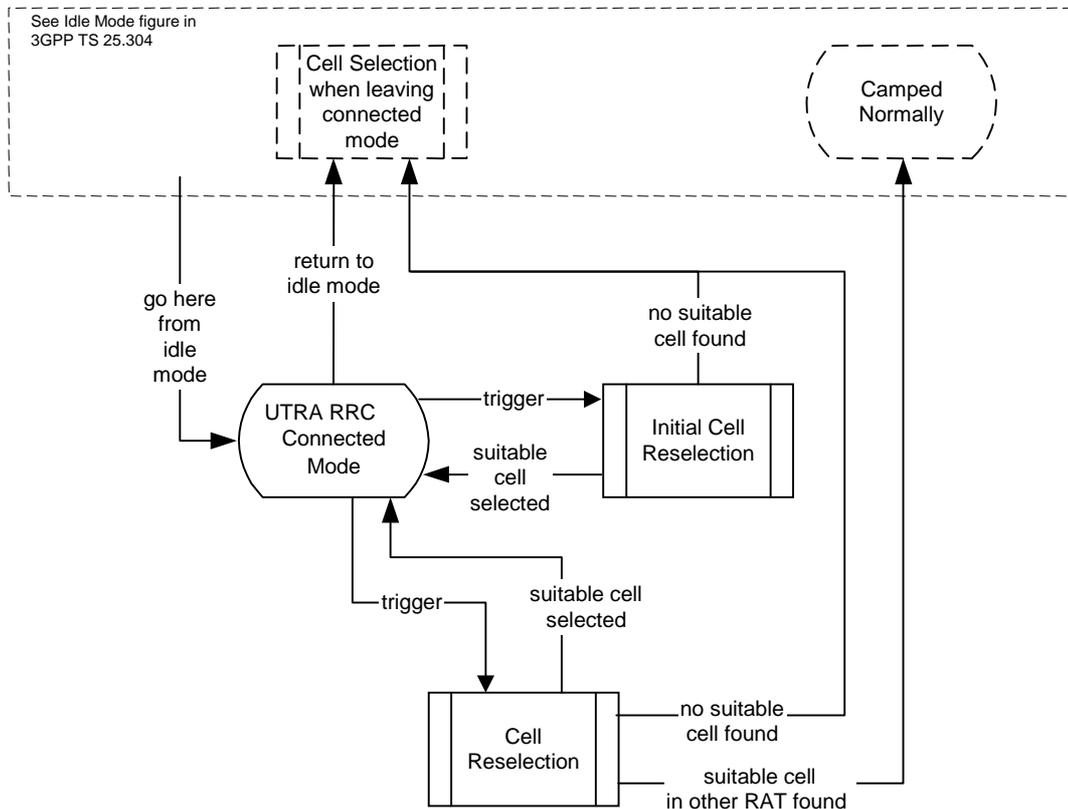
**Figure B.3.5-1: UTRA RRC Connected mode cell reselection for URA\_PCH, CELL\_PCH, and CELL\_FACH**
