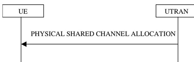
**Figure 8.2.7-1: Physical Shared Channel Allocation**
