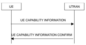
Figure 8.1.6-1: Transmission of UE capability information, normal flow
