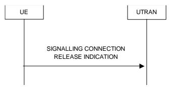
Figure 8.1.14-1: Signalling connection release indication procedure, normal case
