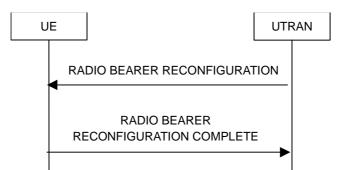
Figure 8.2.2-3: Radio bearer reconfiguration, normal flow
