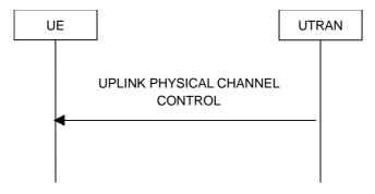
Figure 8.2.10-1: Uplink Physical Channel Control
