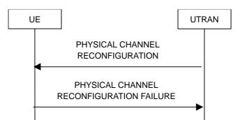
Figure 8.2.2-10: Physical channel reconfiguration, failure case
