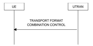
Figure 8.2.5-1: Transport format combination control, normal flow
