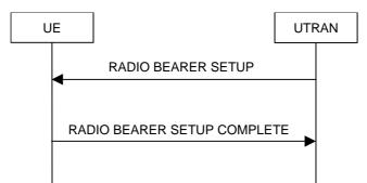
Figure 8.2.2-1: Radio Bearer Establishment, normal case
