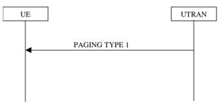
Figure 8.1.1-2: Notification of system information modification for UEs in idle mode, CELL\_PCH state and URA\_PCH state
