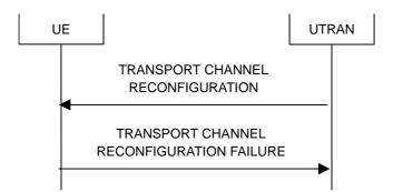
Figure 8.2.2-8: Transport channel reconfiguration, failure case
