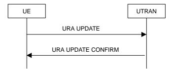
Figure 8.3.1-8: URA update procedure, basic flow
