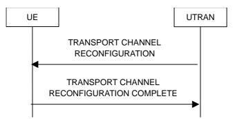
Figure 8.2.2-7: Transport channel reconfiguration, normal flow
