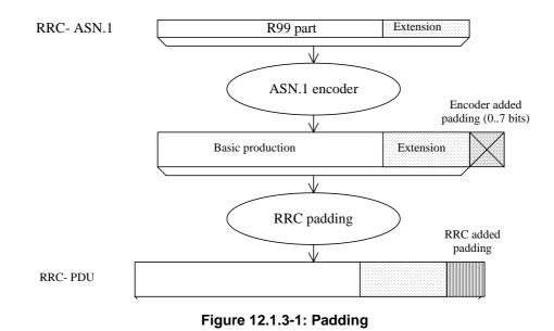
When using AM or UM mode, RLC requires that the RRC PDU length is a multiple of 8 bits.
