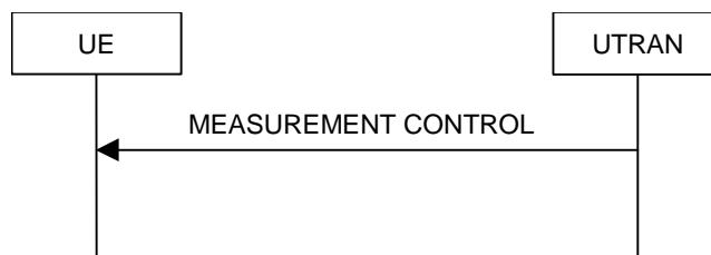
**Figure 8.4.1-1: Measurement Control, normal case**
