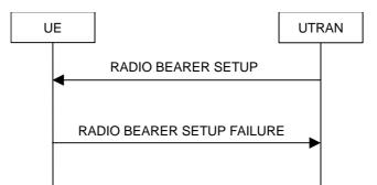
Figure 8.2.2-2: Radio Bearer Establishment, failure case
