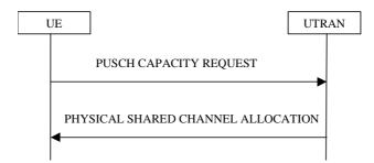
Figure 8.2.8-1: PUSCH Capacity request procedure
