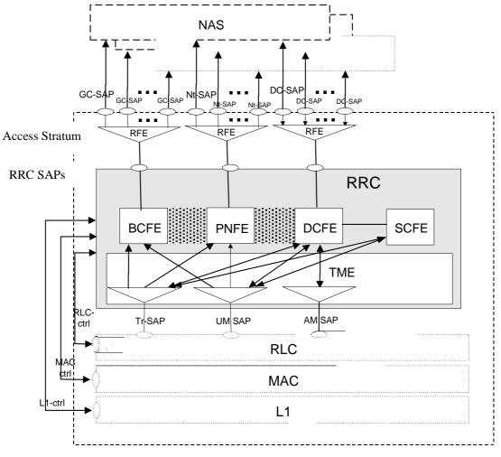
Figure 4.2-1: UE side model of RRC
