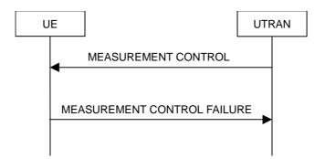
Figure 8.4.1-2: Measurement Control, failure case
