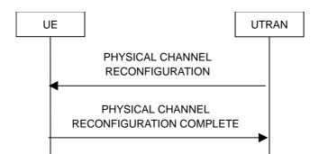
Figure 8.2.2-9: Physical channel reconfiguration, normal flow
