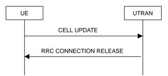
Figure 8.3.1-7: Cell update procedure, failure case
