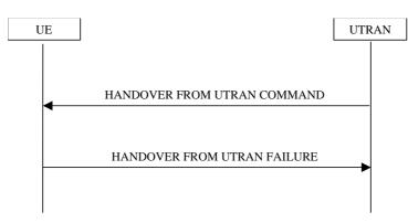
Figure 8.3.7-2: Inter-RAT handover from UTRAN, failure case
