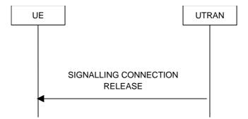
Figure 8.1.13-1: Signalling connection release procedure, normal case
