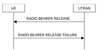
Figure 8.2.2-6: Radio Bearer Release, failure case
