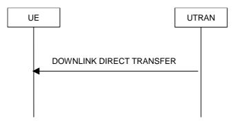
Figure 8.1.9-1: Downlink Direct transfer, normal flow
