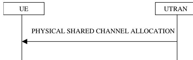
**Figure 8.2.7-1: Physical Shared Channel Allocation**
