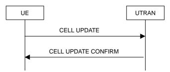
Figure 8.3.1-1: Cell update procedure, basic flow
