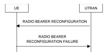
Figure 8.2.2-4: Radio bearer reconfiguration, failure case
