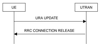
Figure 8.3.1-10: URA update procedure, failure case
