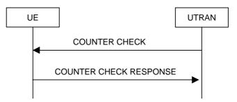
Figure 8.1.15-1: Counter check procedure
