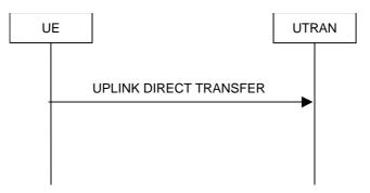
Figure 8.1.10-1: Uplink Direct transfer, normal flow
