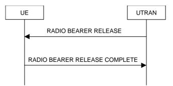
Figure 8.2.2-5: Radio Bearer Release, normal case
