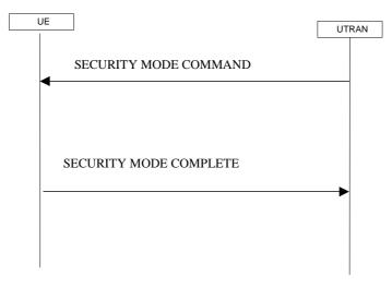
Figure 8.1.12-1: Security mode control procedure
