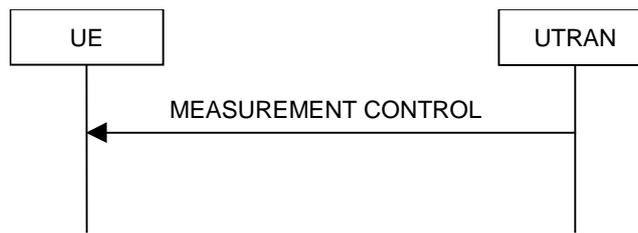
Figure 8.4.1-1: Measurement Control, normal case
