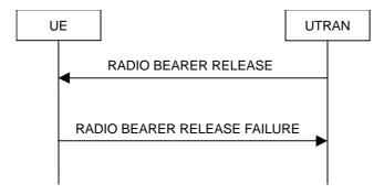
Figure 8.2.2-6: Radio Bearer Release, failure case
