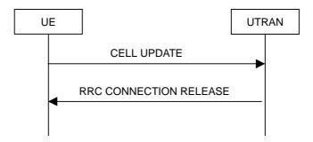
Figure 8.3.1-7: Cell update procedure, failure case
