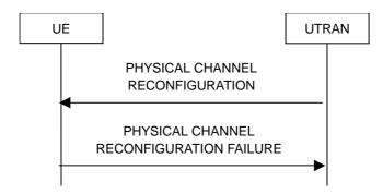
Figure 8.2.2-10: Physical channel reconfiguration, failure case
