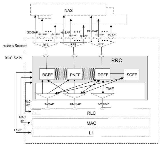
Figure 4.2-1: UE side model of RRC
