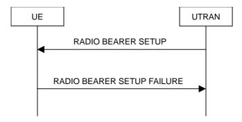
Figure 8.2.2-2: Radio Bearer Establishment, failure case
