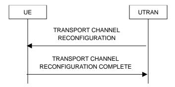
Figure 8.2.2-7: Transport channel reconfiguration, normal flow
