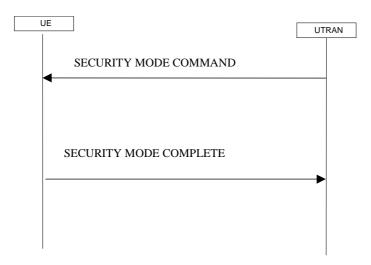
Figure 8.1.12-1: Security mode control procedure
