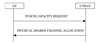
Figure 8.2.8-1: PUSCH Capacity request procedure
