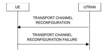
Figure 8.2.2-8: Transport channel reconfiguration, failure case
