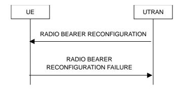
Figure 8.2.2-4: Radio bearer reconfiguration, failure case
