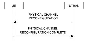
Figure 8.2.2-9: Physical channel reconfiguration, normal flow
