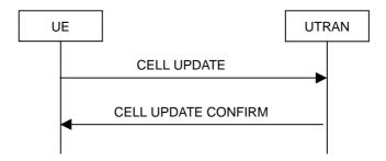
Figure 8.3.1-1: Cell update procedure, basic flow
