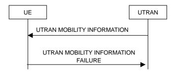
Figure 8.3.3-2: UTRAN mobility information procedure, failure case
