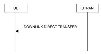
Figure 8.1.9-1: Downlink Direct transfer, normal flow
