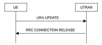
Figure 8.3.1-10: URA update procedure, failure case
