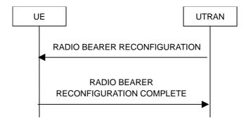
Figure 8.2.2-3: Radio bearer reconfiguration, normal flow
