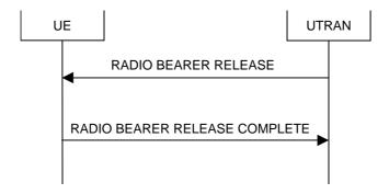
Figure 8.2.2-5: Radio Bearer Release, normal case
