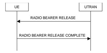
Figure 8.2.2-5: Radio Bearer Release, normal case
