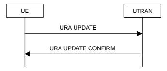
Figure 8.3.1-8: URA update procedure, basic flow
