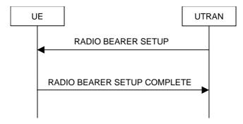
Figure 8.2.2-1: Radio Bearer Establishment, normal case
