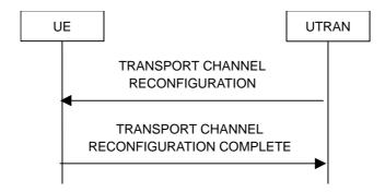
Figure 8.2.2-7: Transport channel reconfiguration, normal flow
