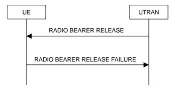
Figure 8.2.2-6: Radio Bearer Release, failure case
