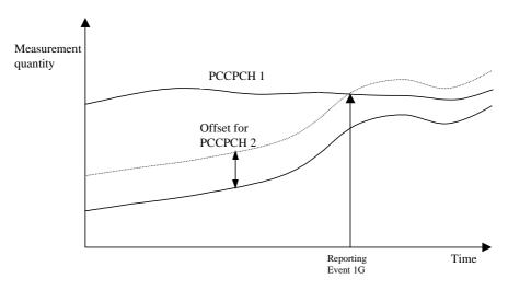
Figure 14.1.5.3-2: A positive offset is applied to primary CCPCH 2
