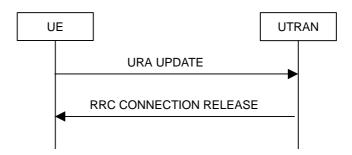
Figure 8.3.1-10: URA update procedure, failure case
