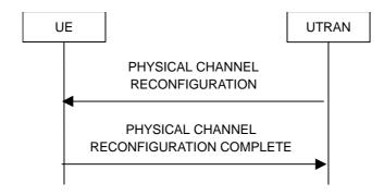
Figure 8.2.2-9: Physical channel reconfiguration, normal flow
