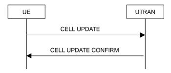
Figure 8.3.1-1: Cell update procedure, basic flow
