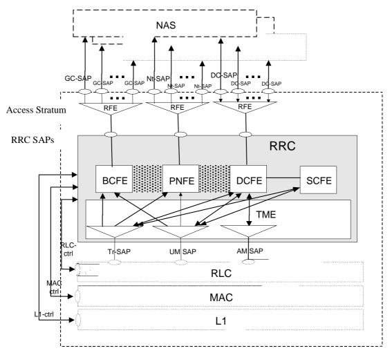
Figure 4.2-1: UE side model of RRC
