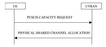
Figure 8.2.8-1: PUSCH Capacity request procedure
