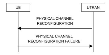
Figure 8.2.2-10: Physical channel reconfiguration, failure case
