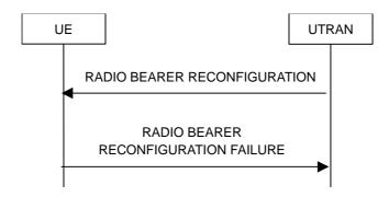
Figure 8.2.2-4: Radio bearer reconfiguration, failure case
