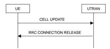
Figure 8.3.1-7: Cell update procedure, failure case
