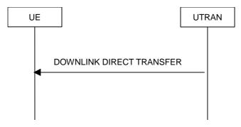
Figure 8.1.9-1: Downlink Direct transfer, normal flow
