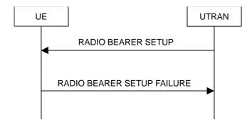
Figure 8.2.2-2: Radio Bearer Establishment, failure case
