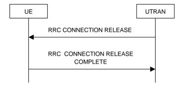
Figure 8.1.4-1: RRC Connection Release procedure on the DCCH
