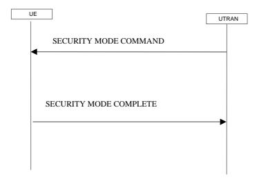
Figure 8.1.12-1: Security mode control procedure
