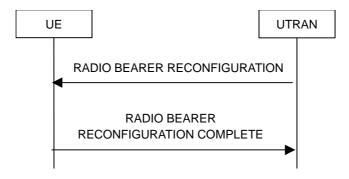
Figure 8.2.2-3: Radio bearer reconfiguration, normal flow
