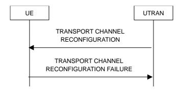
Figure 8.2.2-8: Transport channel reconfiguration, failure case
