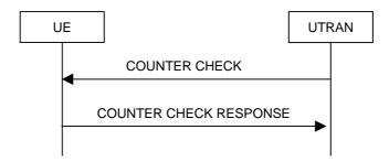
Figure 8.1.15-1: Counter check procedure
