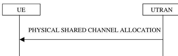
**Figure 34: Physical Shared Channel Allocation**
