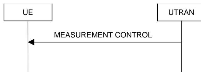
Figure 56: Measurement Control, normal case
