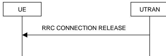
**Figure 11: RRC Connection Release procedure on the CCCH**
