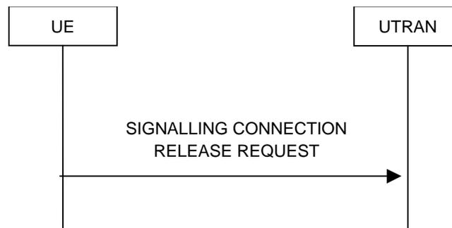
**Figure 20: Signalling connection release request procedure, normal case**
