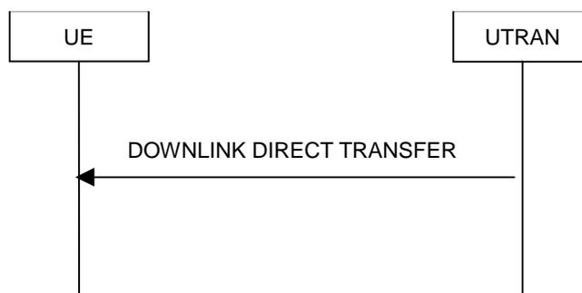
Figure 15: Downlink Direct transfer, normal flow
