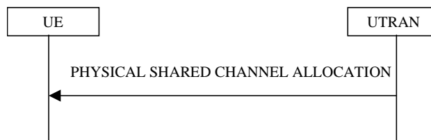
Figure 35: Physical Shared Channel Allocation
