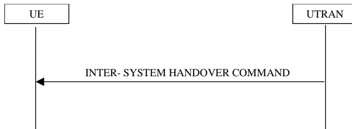
Figure 53: Inter system handover from UTRAN, successful case
