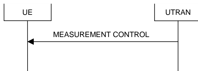
Figure 55: Measurement Control, normal case
