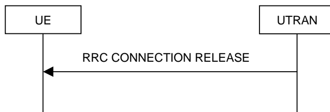
Figure 10: RRC Connection Release procedure on the CCCH
