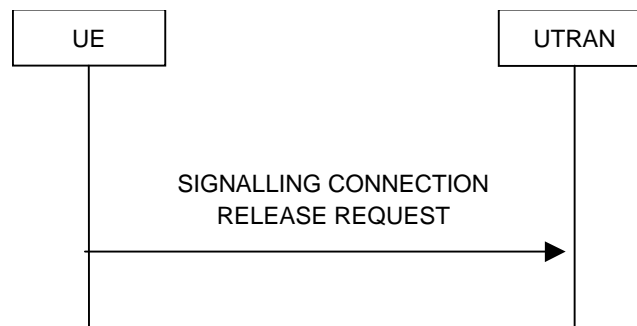
Figure 21: Signalling connection release request procedure, normal case
