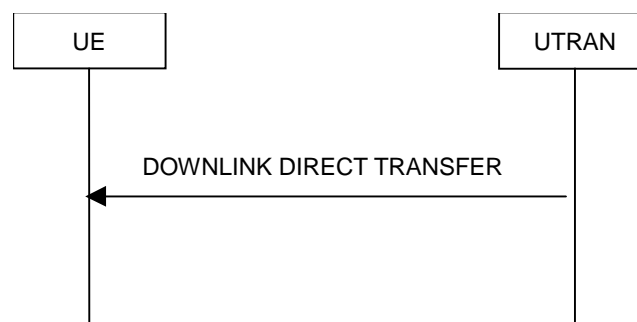
Figure 16: Downlink Direct transfer, normal flow
