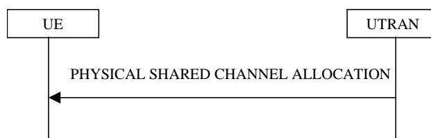
Figure 29: Physical Shared Channel Allocation
