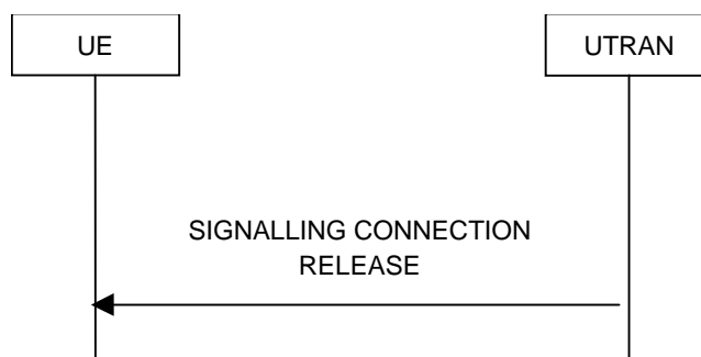
Figure 17: Signalling connection release procedure, normal case
