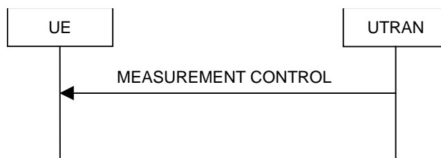
Figure 43: Measurement Control, normal case
