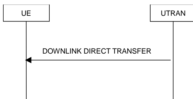
Figure 14a: Downlink Direct transfer, normal flow
