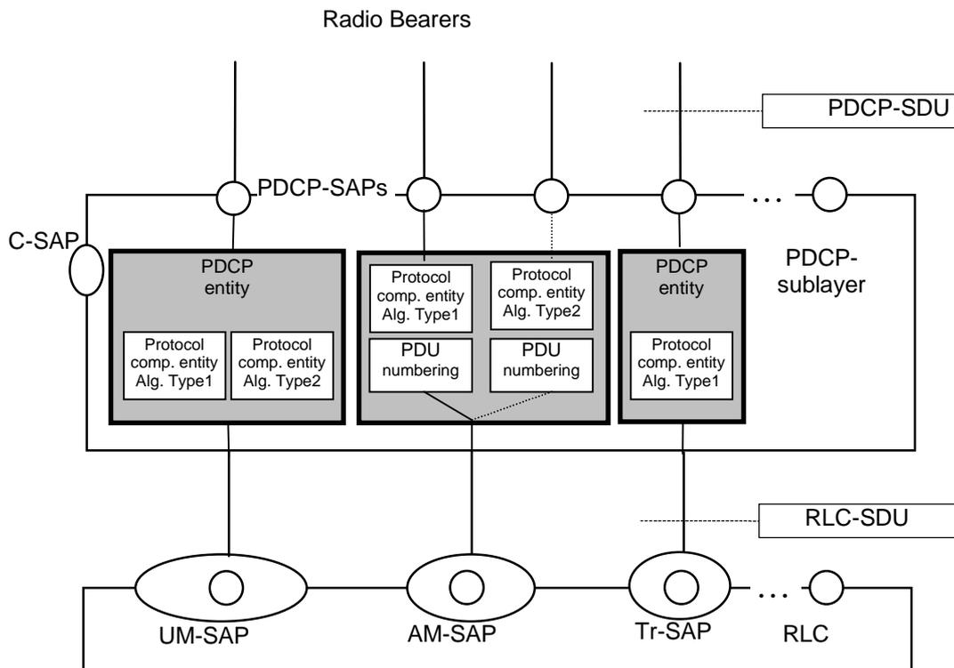
Figure 1: PDCP structure
