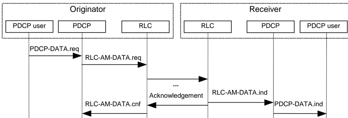
**Figure 2: PDCP data transfer over acknowledged mode RLC**
