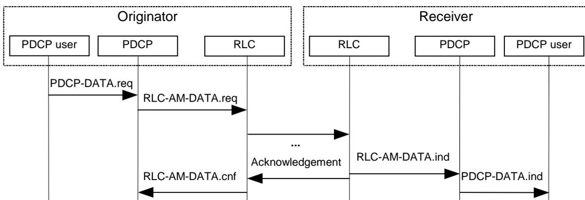
**Figure 2: PDCP data transfer over acknowledged mode RLC**
