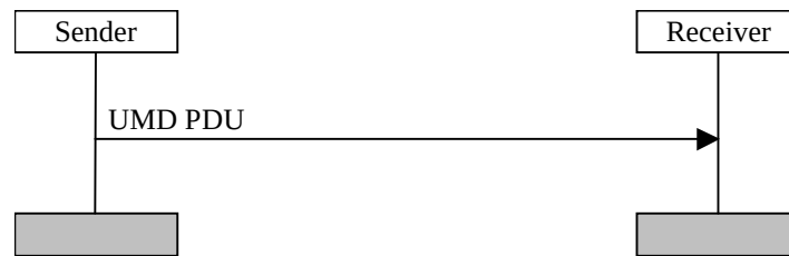
Figure 11.2: Unacknowledged mode data transfer procedure
