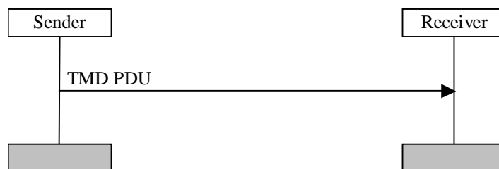
Figure 11.1: Transparent mode data transfer procedure
