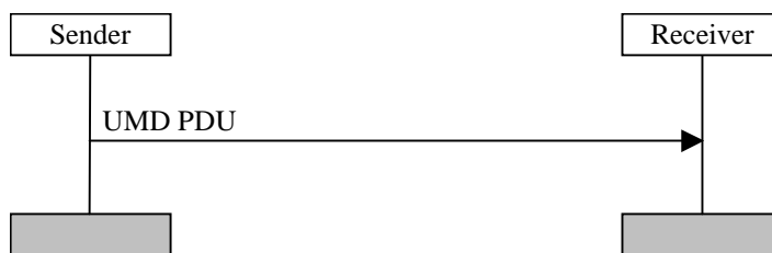
Figure 11.2: Unacknowledged mode data transfer procedure
