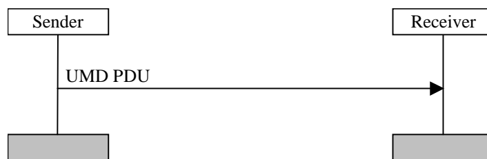
Figure 11.2: Unacknowledged mode data transfer procedure
