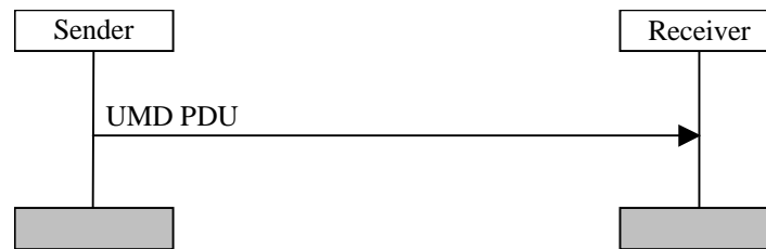
Figure 11.2: Unacknowledged mode data transfer procedure
