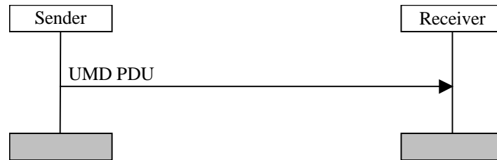
Figure 11.2: Unacknowledged mode data transfer procedure
