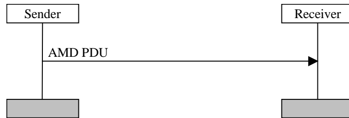
Figure 11.3: Acknowledged mode data transfer procedure
