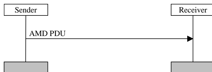
Figure 11.3: Acknowledged mode data transfer procedure
