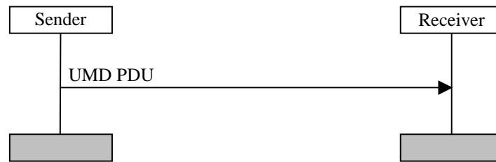
Figure 11.2: Unacknowledged mode data transfer procedure
