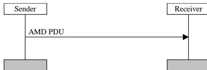
Figure 11.3: Acknowledged mode data transfer procedure
