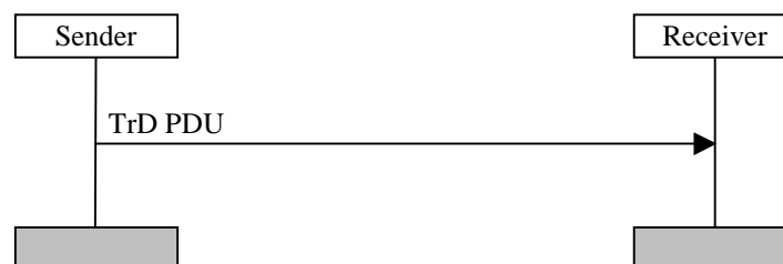
Figure 11.1: Transparent mode data transfer procedure
