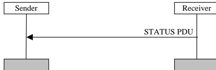
**Figure 11.5: STATUS PDU transfer procedure**
