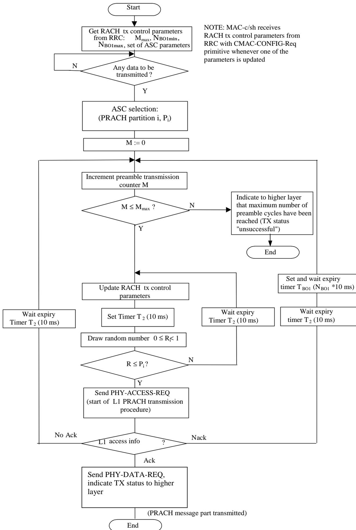
Figure 11.2.2-1: RACH transmission control procedure (UE side, informative)
