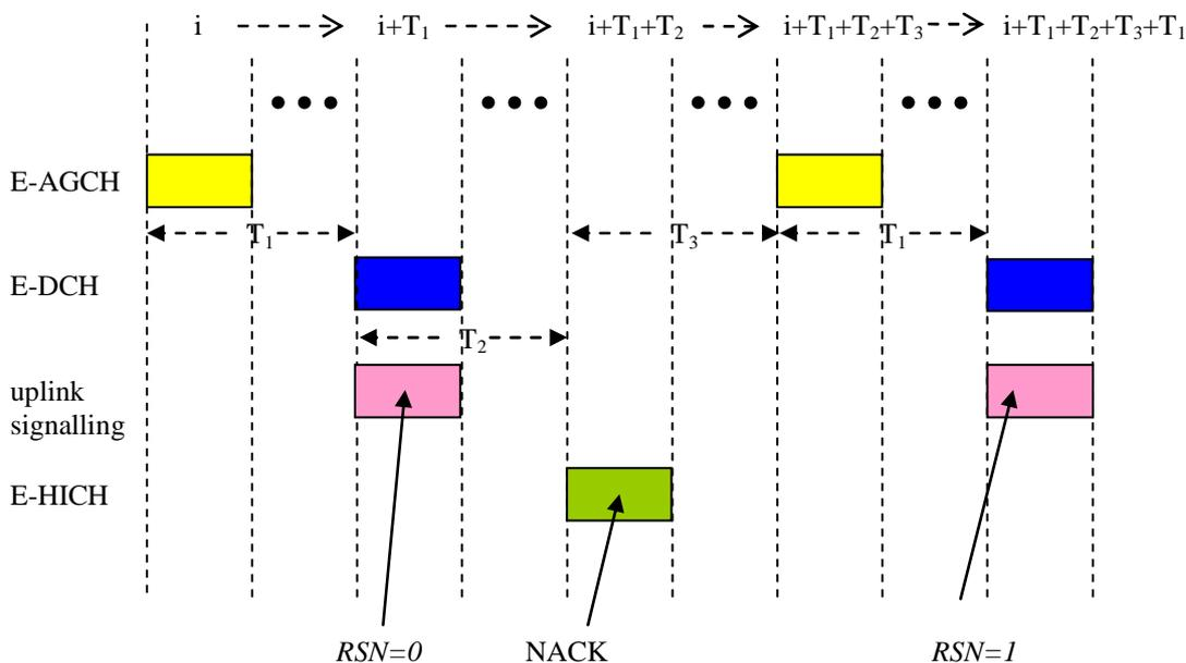
Figure 11.9.1.1-1: TDD E-DCH HARQ Operation
