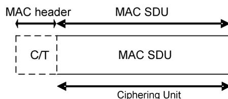
**Figure 11.5-1: Ciphered part unit for a MAC PDU**
