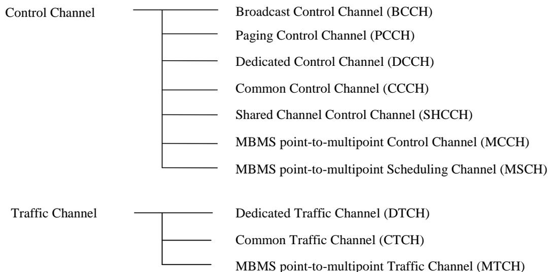
**Figure 4.3.2.1-1: Logical channel structure**
