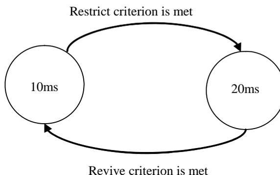
**Figure 11.4.1-1: Transmission Mode Switching transitions for a given TFC**
