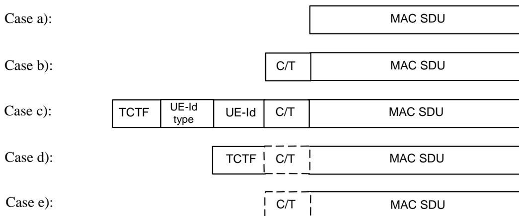
Figure 9.2.1.1-1: MAC PDU formats for DTCH and DCCH
