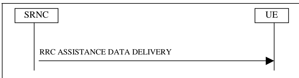
Figure 6.2b: OTDOA or GNSS Assistance Data Delivery Flow
