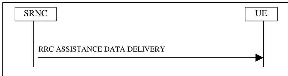
Figure 6.2: OTDOA or GPS Assistance Data Delivery Flow
