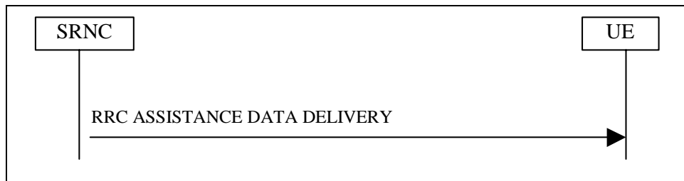
Figure 6.2: OTDOA or GPS Assistance Data Delivery Flow
